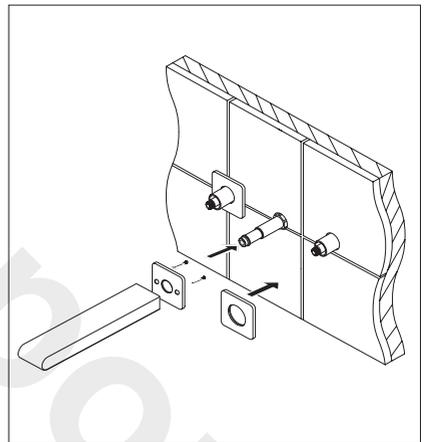
6. Push the plinths onto the valve shrouds and secure by tightening the grub screws.
