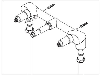
4. Attach the supply pipework to the hot and cold inlets (hot on the left and cold on the right when viewed from the front) ensuring the olive is fitted to the copper pipe work. Tighten the compression nut to secure the pipework and create a water tight seal.
